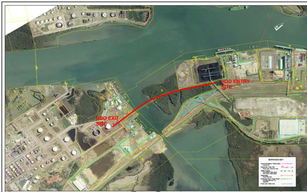
CRUDE & BUNKER PIPELINE REPLACEMENT PROJECT BOREHOLE ALIGNMENT
